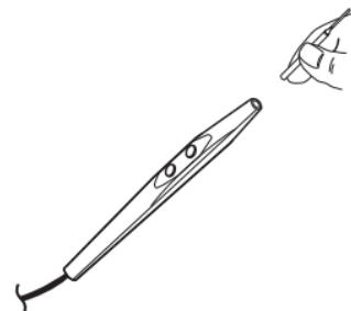
3. Ensure the insulating sleeve fits securely inside the nose of the pencil so that the nose overlaps the insulating sleeve by at least 1/8" (0.3 cm).
